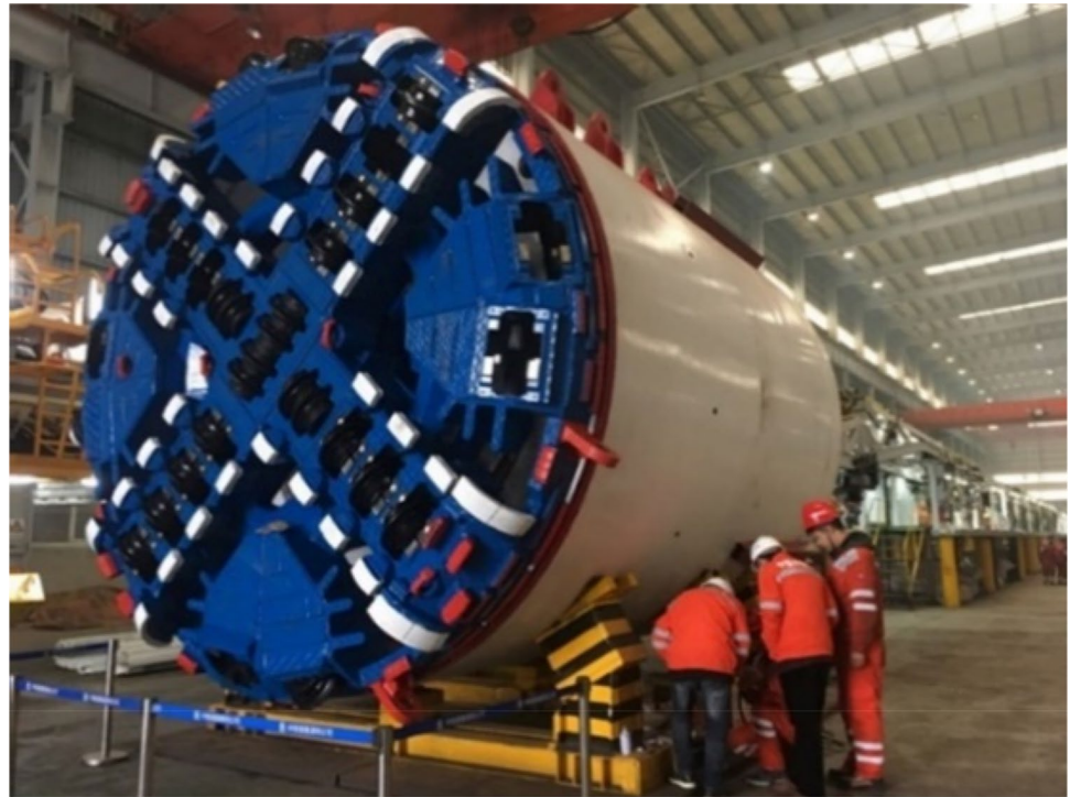
Fig. 16 Earth pressure balanced shield TBM
